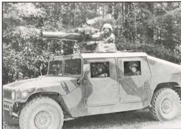
This Highly Mobile Motor Wheeled Vehicle (HMMWV), known as the "humvee," is one of 225 used in the Maryland Army National Guard as a replacement for the popular and long-used 1/4-ton jeep and can be used for tactical and medical purposes.
