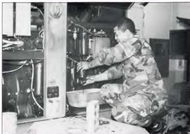
KEEPING IT RUNNING: Sgt. Willie Lyle, Combined Surface Maintenance Shop, Maryland Army National Guard, changes the oil on a 60 kw generator. (Photo by Lt. Col. James Degatina)
