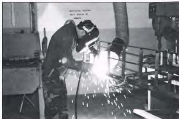
DANGEROUS DUTY: Sparks fly as Sgt. Kent Meadows, 1729th Maintenance Battalion, Maryland Army National Guard, gives his protective equipment a workout as he welds a Humvee brush guard. (Photo by Lt. Col. James Degatina)
