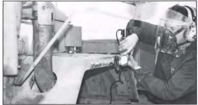
DOWN TO THE METAL: Staff Sgt. Curtis J. Meadows, assigned to the Surface Maintenance Office in Havre de Grace, grinds a rusted area on 2 ½ ton truck. (Photo by Lt. Col. James Degatina)
