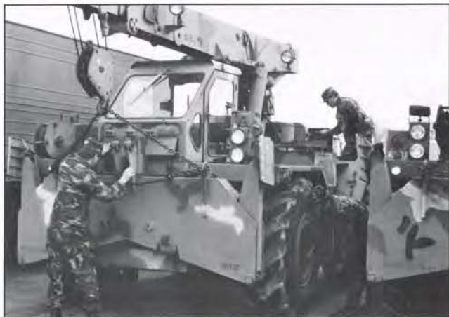
TIE-DOWN: Staff Sgt. John Seaver, 1729th Maintenance Company, Maryland Army National Guard, right, and another soldier secure a 7 1/2-ton crane before taking it on the road. (Photo by Lt. Col. James Degatina)
