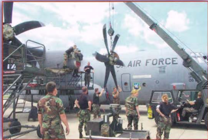
Ground crews change propellers on a C130J at Warfield Air National Guard Base
