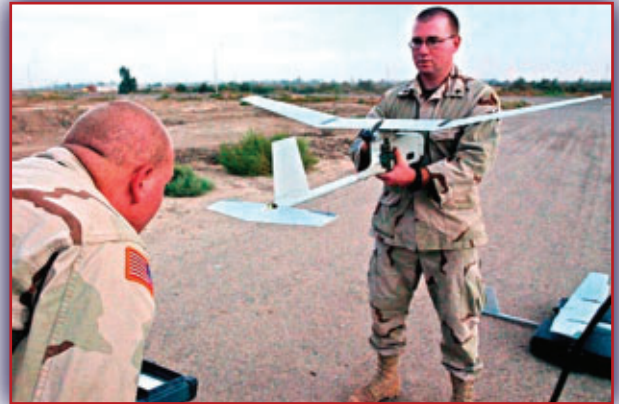
Members of the 629th Military Intelligence Battalion perform pre-flight checks on a Raven Unmanned Aerial Vehicle while in Iraq. (U.S. Army photo by Cpl. Benjamin Cossel)
