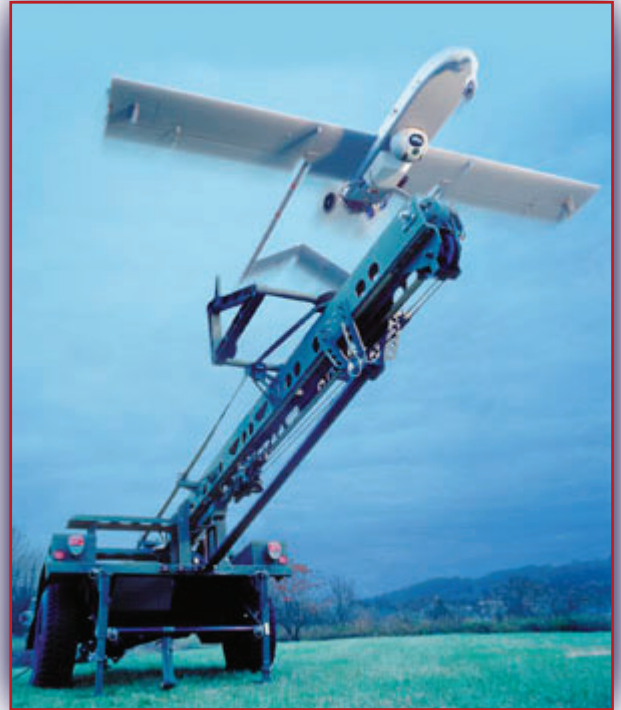
The Tactical Unmanned Aerial Vehicle (TUAV) system manufactured by AAI Corporation of Hunt Valley, Md., is designed as a ground maneuver commander's primary day/night reconnaissance, surveillance, target acquisition, and battle damage assessment system. The 629th Military Intelligence Battalion is one of the first National Guard units to receive this latest technology in the Global War on Terror.
