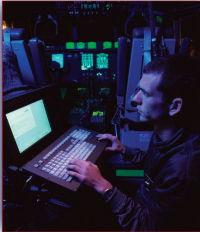
Staff Sgt. Peter J. Ramsey, 135th Maintenance Squadron, uses the computerized Portable Maintenance Aid to diagnose potential problems with the computerized C-130J.
