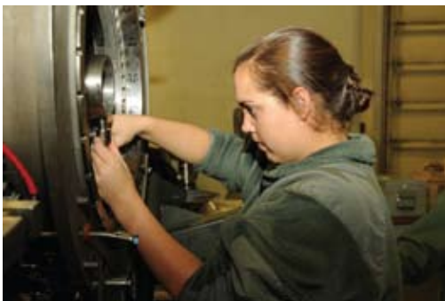
Staff Sgt. Leslie Ranlet works on High Pressure Turbine run outs. (Photo by Tech. Sgt. Chris Schepers.)
