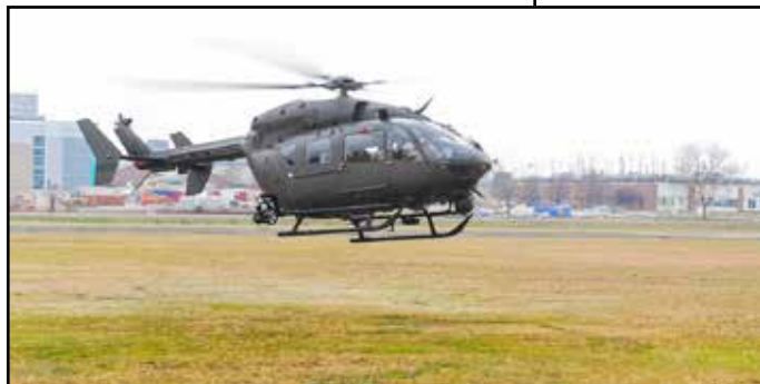
A Maryland National Guard Counterdrug LUH-72 Lakota helicopter returns from a mission. This is the U.S. Army's newest light utility helicopter, replacing the older OH-58 Kiowa helicopters.
